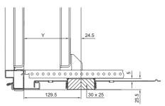
Y = Mounting plate depth-adjustable on a 25 mm pitch pattern (final pitch 30 mm)
